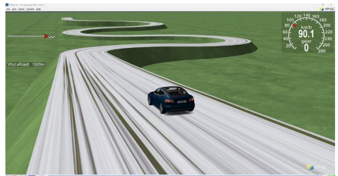
Figure 8. Test vehicle on snowy road using the CarMaker IPG Movie function
