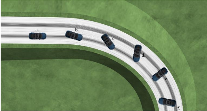
Figure 14. Vehicle dynamics during recuperation fault injection on snowy road
